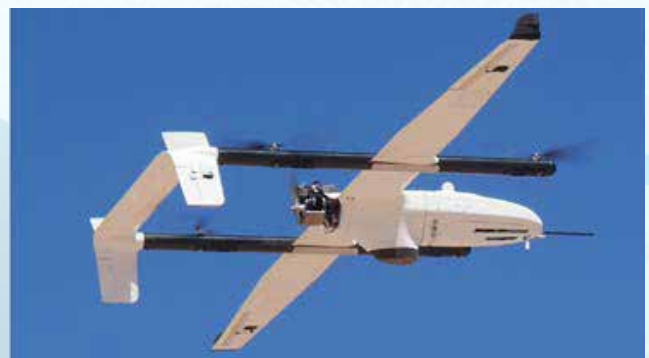
The L3 Latitude is a hybrid quadrotor UAS that combines vertical takeoff and landing with the speed and range of a fixed-wing aircraft. NOAA is testing it for launching from a ship for climate and air quality studies, fishery and mammal surveys, weather observations, oil spill detection, and post severe weather damage assessments. Photo credit: NOAA PMEL/Trish Quinn.
