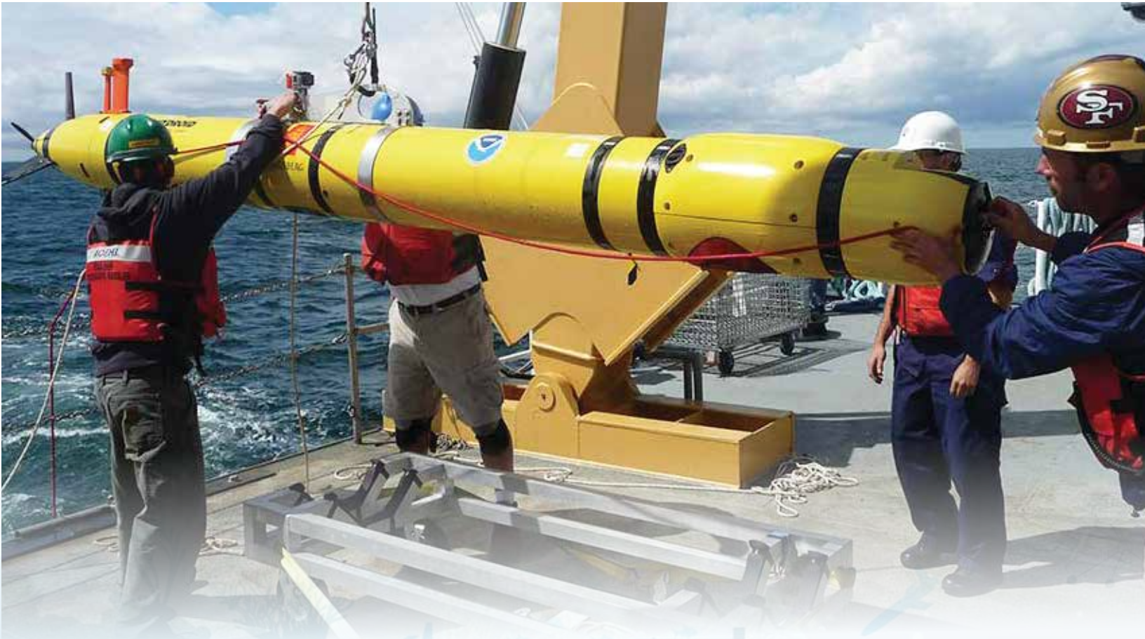
NOAA Ship Ferdinand R. Hassler crew recover the Office of Coast Survey's Hydroid REMUS 600 UUV after completion of a bathymetric mapping mission. This vehicle can operate for 20+ hours at depths up to 450 meters while maintaining acoustic communications with the host ship. Photo credit: NOAA/OCS.
