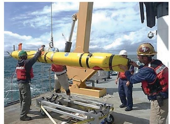
NOAA's Office of Coast Survey prepares to launch a Hydroid REMUS 600 autonomous underwater vehicle on a bathymetric mapping mission. This vehicle can operate for 20+ hours at depths up to 450 meters while maintaining acoustic communications with the host ship.
