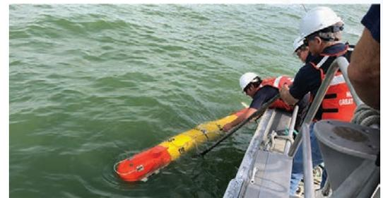
For the third year in a row, NOAA is using Environmental Sample Processors designed by the Monterey Bay Aquarium Research Institute and mounted on a UUV to study potentially toxic algal blooms in Lake Erie in collaboration with NOAA's Great Lakes Environmental Research Laboratory.
