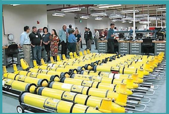
NOAA's Integrated Ocean Observing System partnered with the U.S. Navy and Shell Oil Co. to share data from over 20 gliders deployed in the Gulf of Mexico in 2018. Salinity and temperature data from gliders can improve hurricane intensity forecasts.
